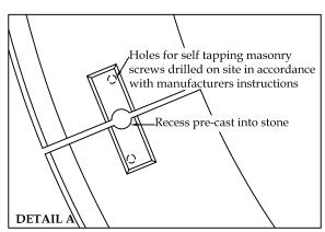
Read in conjunction with Tech Sheet P10, P20, P30, P60 and P80 All dimensions exclude joints - allow 6mm  $(\frac{1}{4})$  for vertical and bedding joints Unless otherwise stated, all materials other than stonework to be supplied by others
